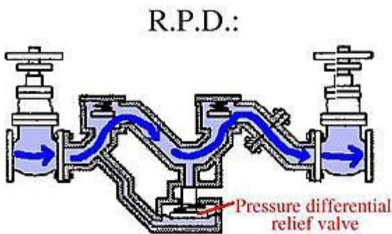
Reduced Pressure Zone (or device) is a highly sensitive and efficient backflow protector designed to protect a water system or facility from what is referred to as high hazards. RPZ's have two (2) check valves and then one differential relief valve in the middle. When a backflow occurs the relief valve opens to allow air in to “break” the vacuum created. This device will continue to work even if one or both check valves are compromised.
